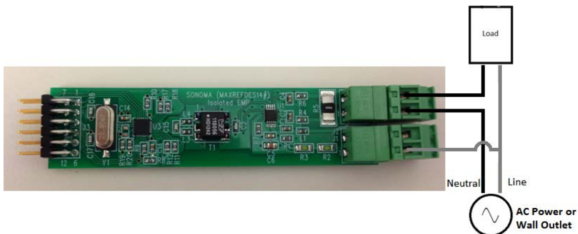
Figure 4. Sonoma Power and Load Connections
